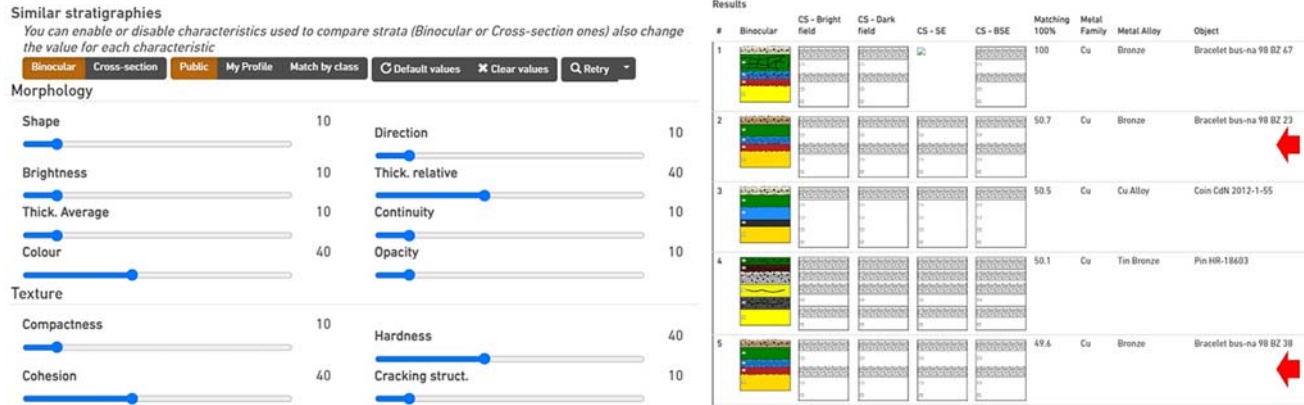
Figure 2.3.3 Result of the (by default) MiCorr database query for the binocular stratigraphy in Fig. 2.3.2c. On the left, the subcharacteristics values filled in (in blue, detail). On the right, the matching proposals of the database: the stratigraphy under binocular mode, the matching %, and the information on the corresponding metal, alloy and object (detail).
